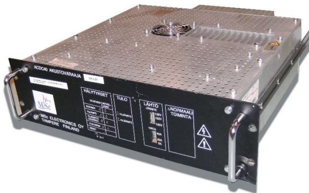
Battery Charger located inside the coach.
