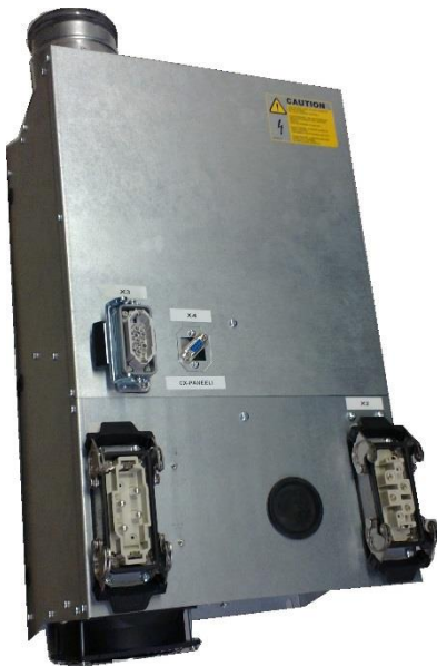
Power Converter for the air conditioning unit is located inside the coach
